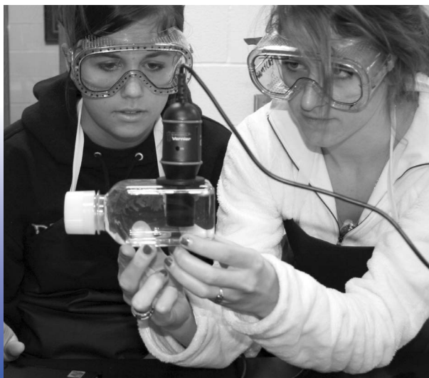
Using an oxygen gas sensor, students are measuring the oxygen level in water samples at different temperatures.
